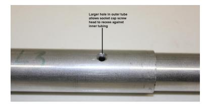
Each tube has one larger, counterbored hole drilled on one end, on one side. **The side of the tube with the counterbored hole is ALWAYS the outer tube of a joint, with the smaller outer-diameter tube sleeved inside.**
