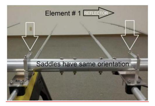
Before final torquing, re-check spacing and horizontal alignments of element center sections on the boom using the measurements illustrated on Diagram 1.
