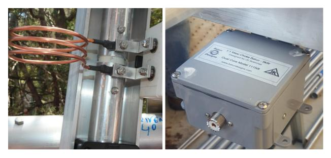
5) Check the entire setup for snug fit and make sure there are no loose joints in the coil or the balun leads.
