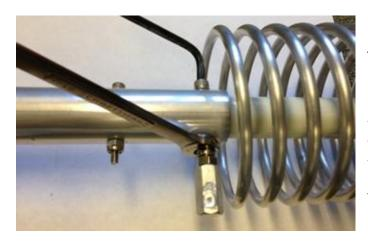
**NOTE:** It is very important to have a solid mechanical connection, with the nut and screw making a tight contact over the tubing. Visually inspect the coil assembly for any twists or non-symmetry while tightening these nuts. Adjust them carefully by pulling them back into place. Repeat this same process for all the coil assemblies.
