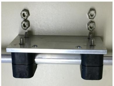
Element being mounted to Element Plate using Black Clamps and nylon nuts
