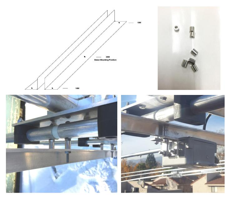
The JK MIDTRI is delivered without a balun. We recommend a 1:1 current balun since the antenna is designed to be fed with a 50 Ohm balanced source, bringing the antenna to true optimum performance.
