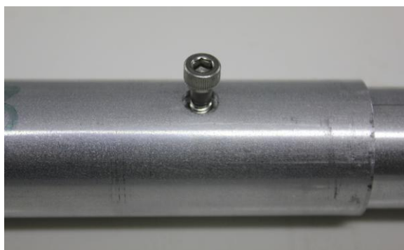
Screw fits into recessed hole - face up
