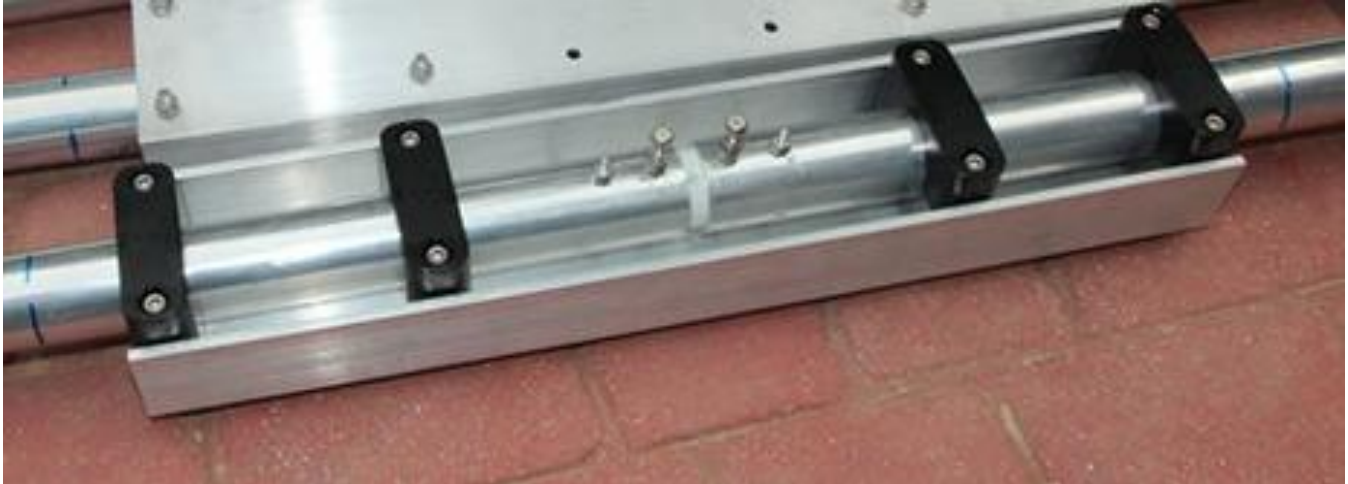
40M center sections mounted on element channels
